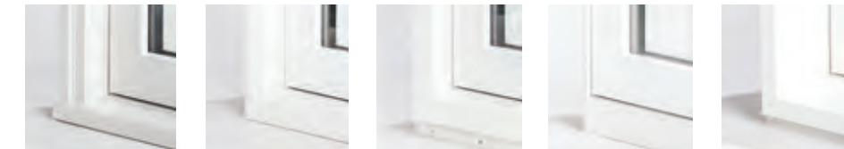
2" brickmould on all sides or with sloped sill. Mirrors the look of wood windows 1 1/2" brickmould on all sides for a slimmer appearance 1 1/2" HD brickmould with nail fin. J-trim version available Handy rebate flange to cover existing material 3/4" exterior extender pushes the window back, creating a shadow box. Also ideal for ICF
